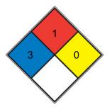
Short exposure could cause serious temporary or moderate residual injury (e.g. <u>liquid hydrogen, sulfuric acid, calcium</u> HEALTH 3 <u>hypochlorite</u>, hexafluorosilicic acid)
