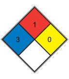
Short exposure could cause serious temporary or moderate residual injury (e.g. <u>liquid hydrogen, sulfuric acid, calcium</u>
